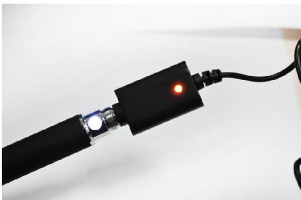
2. The light on the charger will turn red as shown above indicating that the battery is now being charged.
