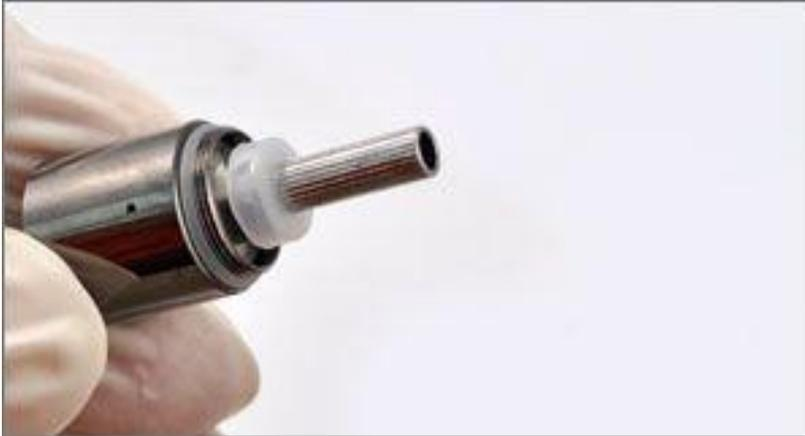
2. Unscrew the Coil from the base and replace with a new one. Replacement Coils can be purchased separately.
